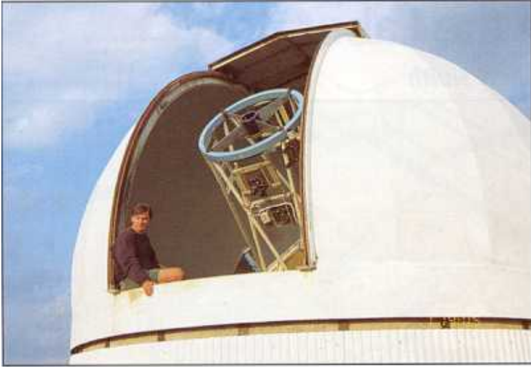
Dany Cardoen and the 1m telescope. The ST-4 autoguider is visible on the Serrurier truss mount. The Newtonian focus was available at any of four positions.
