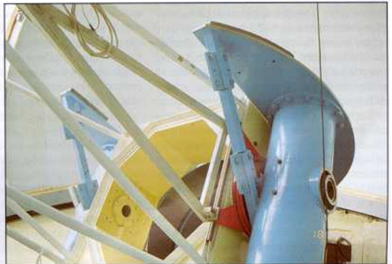
The mount of the 1m telescope. The red declination tangent arm can be seen next to the yellow mirror box. The declination axis is hollow to allow installation of a Nasmyth focus.
